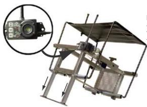
An extension leg is provided if you require an angled launch. This can prove valuable in forcing the bird to fly in a predetermined direction. Position the launcher where you want the bird to be released. Press the button snap and pull down on the extension bracket until it locks into place.
