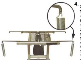
\*Connect the springs one at a time in this sequence. Loop one end of the spring through each end of the metal arm assembly. Repeat with the opposite spring. The springs should be dangling loose. NOTE: This Launcher can be operated using only 2 springs. Using all four springs requires considerable strength to load and reduces spring life due to the extra stress exerted at launch.
