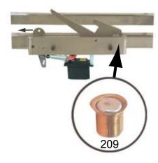
2. Grasp both metal arms and force downward. The pouch will drop into the frame of the launcher as the swing arm engages the release arm. Push downward until you see and hear the trigger and release arm engage each other. IMPORTANT: Keep your force on the metal arms until you are sure that the launcher is cocked. Quickly step away and remove your arms and hands from the danger zone.
