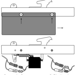
Remove the two bolts that secure the protective shield to the release. Move the shield over to expose the servo and wiring.
