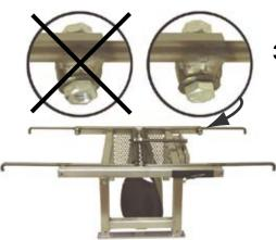
Align the metal arm bushings to the box frame holes and install all 4 bolts and lock nuts. Make sure the bolts are facing inside and the nuts are facing outside. Tighten the bolts so that the metal arms still pivot freely. IMPORTANT: Do not over tighten.
