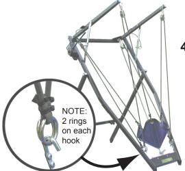
4. Walk around the back of the Winger and repeat Step 3. WARNING: Do not walk in front of the Winger. Serious injury can result if misfire occurs. All four rubbers are now hooked up and the pouch is ready for a bird or bumper.
