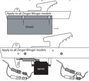
Remove the two bolts that secure the release to the protective housing. Remove the shield to expose the servo and wiring.
