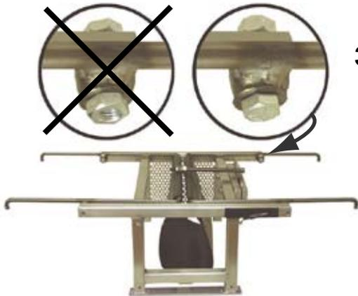
3. Align the metal arm bushings to the box frame holes and install all 4 bolts and lock nuts. Make sure the bolts are facing inside and the nuts are facing outside. Tighten the bolts so that the metal arms still pivot freely. **IMPORTANT: Do not over tighten.**
