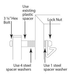
If your Zinger Winger was purchased prior to 2008 your new support hinges will be different than the original equipment. You will need to replace the original 3" Hex bolts with the new bolts and lock nuts that are included with your new hinges.
