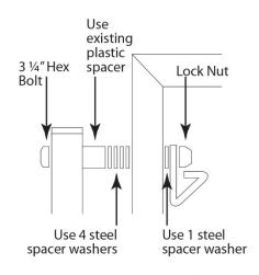
If your Zinger Winger was purchased prior to 2008 your new support hinges will be different than the original equipment. You will need to replace the original 3" Hex bolts with the new bolts and lock nuts that are included with your new hinges.
